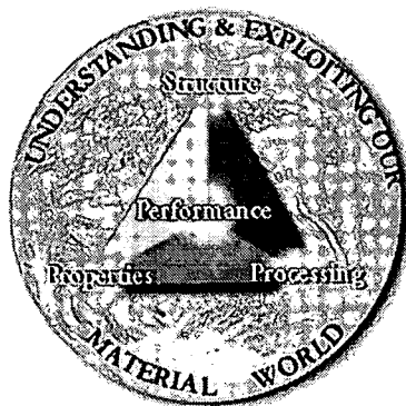
Figure 2: Connections made within each module. A material's atomic structure, properties, processing and performance are all related at the nano-level, as well as the macro-level.
